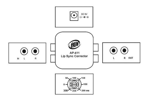
Connect audio inputs from the source equipment to the R and L RCA connectors on the AP-411. Next, connect the AP-411's R and L outputs to the destination equipment.
